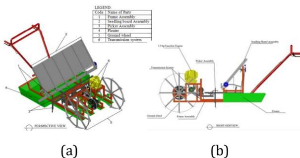
**Figure 1.** Component parts of the self-propelled mechanical rice transplanter (a) perspective view and (b) right side view
